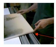
Allow art & wood stretcher to fall forward off of Stretcher Plates
