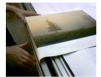
• Move art & wood stretcher toward operator so it aligns with front face of clamp
