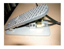
Foot Pedal – Operates "Clamping Bar" (Normally Open)
