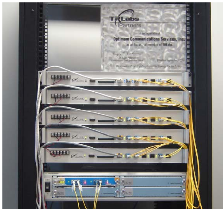
Adaptive-Mesh test network with five ITN nodes and MPLS router tester.
